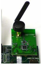
Connect the CC85xxEM or the CC85xx-CC2590EM marked SLAVE (label attached on the backside of the board.) These boards are pre-programmed with slave firmware. Attach the antenna to the SMA connector.
