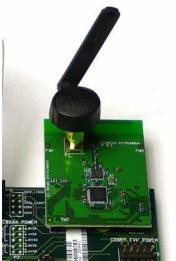
Connect the CC85xxEM or the CC85xx-CC2590EM marked MASTER (label attached on the backside of the board). These boards are pre-programmed with master firmware. Attach the antenna to the SMA connector.
