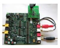
Connect an audio source (CD-player, MP3-player or similar) to the line-in input of the AudioEB with CC85xxEM or CC85xx-CC2590 with the "MASTER" label plugged in.
