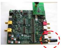
Connect an amplifier to line out or connect a headphone to the mini jack of the AudioEB with the CC85xxEM or the CC85xx-CC2590 with the "SLAVE" label plugged in.
