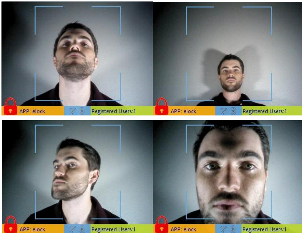
Figure 102: Improper Face Angle & Proximity
