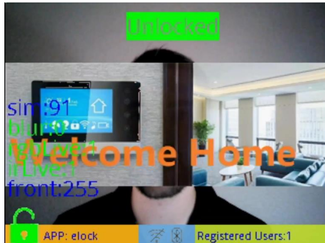
Figure 21: On-screen Info for Recognized Face
