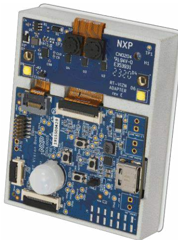
Figure 2: Dual Camera Adapter Kit Configuration
