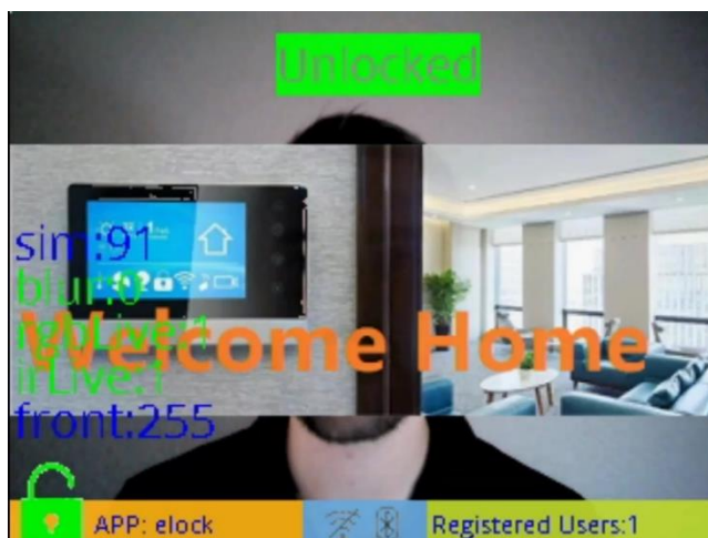
Figure 46: On-screen Info for Recognized Face
