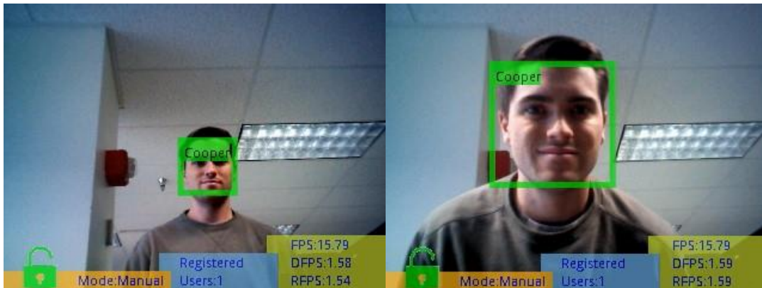
Figure 58: VGA vs. QVGA Detection Resolution Max Range
