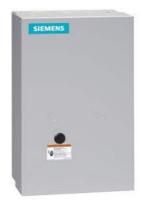
Electrically held lighting contactor, Contactor amp rating 30A, 0 N.C. / 9 N.O. Poles, 347VAC 60HZ coil, Non-combination type, (no disconnect device), Enclosure NEMA type 1, Indoor general purpose use
