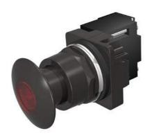
30mm BlackMax, Epoxy Coated Corrosion Resistant Complete Metal Unit Illuminated Push-Pull Operator Full Voltage, 6V AC LED Lamp Mushroom Head Cap Small 1 3/4" (44.5 mm) Metal, Black with Red Lens 3 Position Momentary UL Listed, CSA Certified NEMA 1,3,3R,4,4X,12,13 & Automotive Standards
