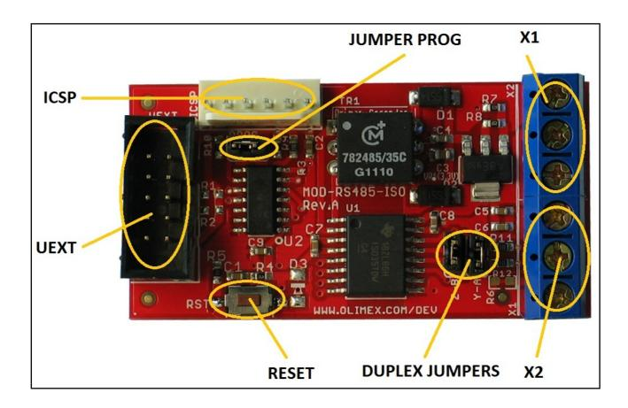
The picture above shows the initial revision of MOD-RS485-ISO. The latest revision features different PIC16 chip.
