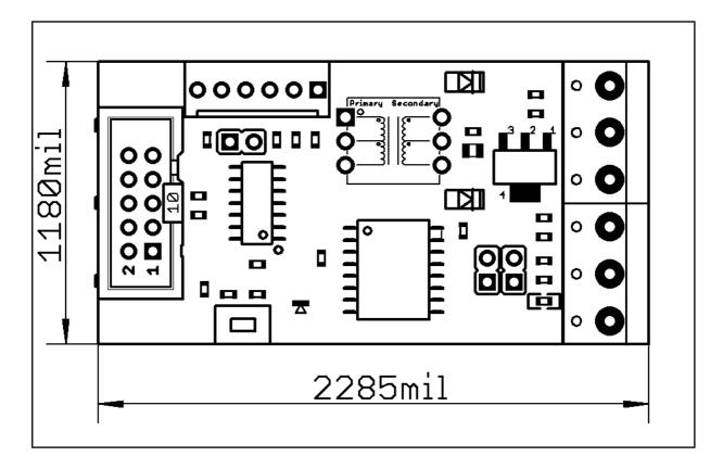
The three highest elements on the board in order from the tallest to the shortest are: ICSP connector – 450mils, RS485 connector – 400mils, UEXT connector – 350mils.
