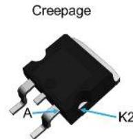
Figure 22. Creepage without top coating
