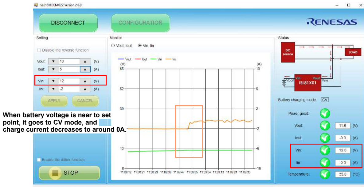
Figure 13. Fully Charging Information in GUI
