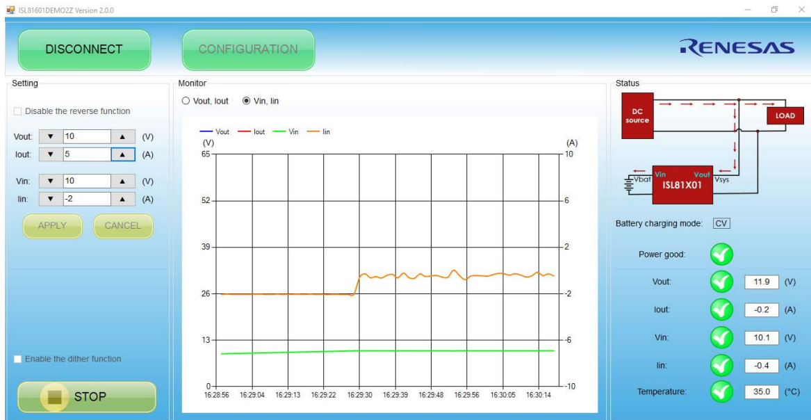
Figure 5. Fully Charged Information in GUI
