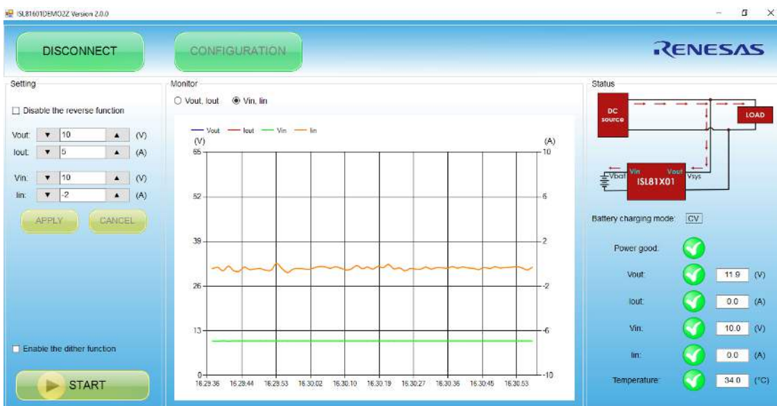
Figure 7. Precharge Complete Information in GUI
