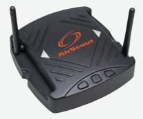
AirScout enables Service Provider technicians with a tool that emulates the complex Wi-Fi<sup>®</sup> home environment enabling technicians with the visibility into the real user experience throughout the home.
