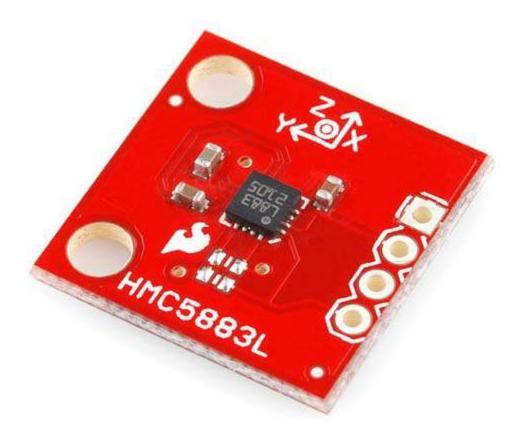
Triple Axis Magnetometer Breakout - HMC5883L
