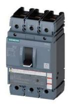
circuit breaker 3VA5 UL frame 250 breaking capacity class C 100kA @ 480 V 3-pole, line protection TM210, FTFM, In=100A overload protection Ir=100A fixed short-circuit protection li=10 x In UL489 SB (naval), 50 deg. cel. nut keeper kit on both sides
