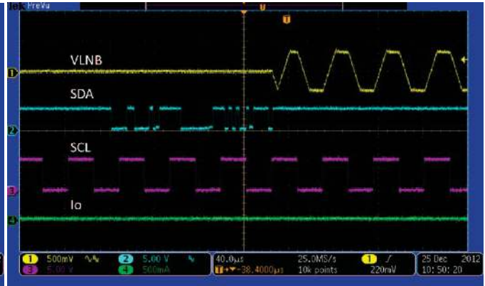
Figure 38. V_{IN} = 12\text{ V} , V_{LNB} = 13.4\text{ V} , No Loading, 22-kHz Tone Delay from I 2 C Gated, EXT M Provides 22 kHz to Output Tone, On
