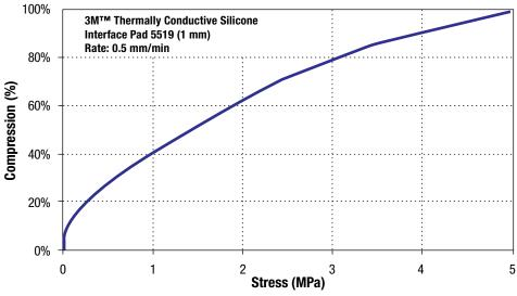
**Note:** Compression vs Stress test results can vary between test methods based on sample size, exact test set-up, equipment type, etc.
