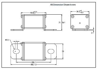
Note: Recommend tightening torque is 12+/-1.0Nm (M8)
