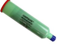
Specifications Alloy: Sn96.5/Ag3.0/Cu0.5 Mesh Size: T5 Micron (µm) Range: 15-25 Flux Type: Synthetic No-Clean Flux Classification: ROL0 Metal Load: 85.75% Metal by Weight 217-220°C (423-428°F) Melting Point: 500g Cartridge Packaging: Shelf Life: Refrigerated >6 months, Unrefrigerated >2 months \*See notes below:
