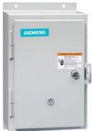
Non-reversing motor starter, Size 1 3/4, Three phase full voltage, Solid-state overload relay, OLRelay amp range 10-40a, 24VAC 50-60HZ coil, Non-combination type, Enclosure type 12, Dust/drip proof for indoors, Extra-wide enclosure
