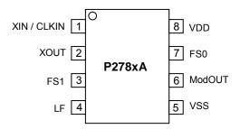
Standard pin Configuration offered in both 8 pin SOIC Packages.
