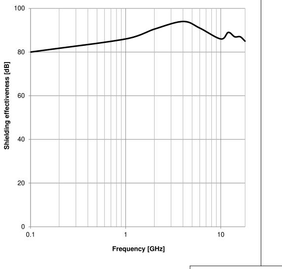
CHECKED REVISION DATE (YYYY-MM-DD) GENERAL TOLERANCE PROJECTION METHOD JoV 005.002 2019-01-01 DIN ISO 2768-1m DESCRIPTION **WE-LT Conductive Shielding** Würth Elektronik eiSos GmbH & Co. KG Gasket ORDER CODE EMC & Inductive Solutions Max-Eyth-Str. 1 3031004 74638 Waldenburg Germany SIZE/TYPE STATUS Tel. +49 (0) 79 42 945 - 0 www.we-online.com BUSINESS UNIT PAGE WÜRTH ELEKTRONIK 2/3 D-Profile eiSos Valid eiSos@we-online.com
