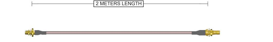
Connector A 132286 SMA Jack Straight Bulkhead - Rear Mount Brass Gold + Heatshrink 50 Ohm RG-178 Continuity/Hi-Pot Connector B 142231 SMB Jack Straight Bulkhead - Rear Mount Brass Gold + Heatshrink
