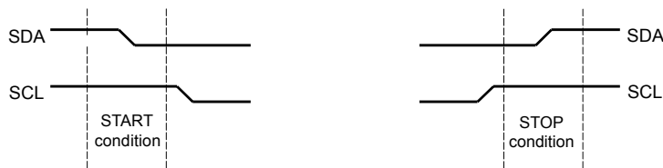
Figure 21-3. START and STOP Conditions
