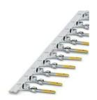
Crimp contact, Pin, rolled, Taped articles, number of pieces per reel: 10000, contact diameter: 1 mm, crimp range: 0.22 mm<sup>2</sup> ... 0.56 mm<sup>2</sup>, Item is lead-free in accordance with RoHS II without Exemption 6c (Pb <0.1%)
