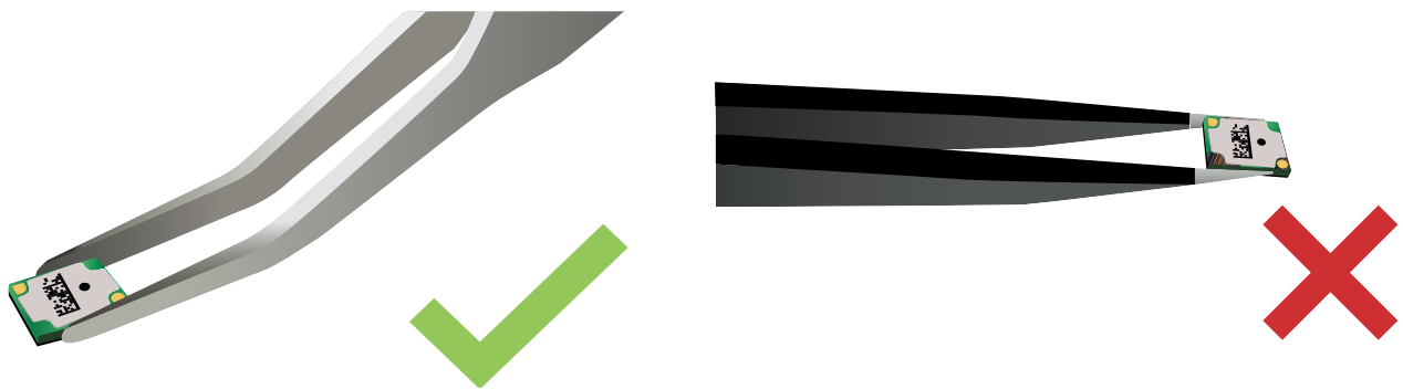
Figure 13: Left: Recommended tweezers type. Right: Not recommended tweezers type
