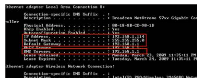
Figure 4: IPconfig on Simple Network
