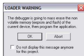
Figure 4: Re-Flashing the chip
