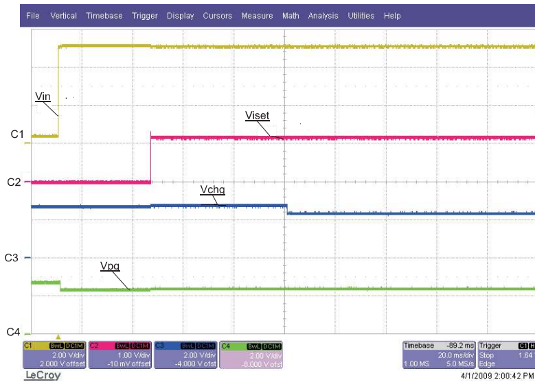
Figure 4. Power-Up Sequence Shows Timing Between Vin, Viset, Vpg, and Vchg. C1: Chg @ JMP1; C4: PG @ JMP8; LEDs Pulled Up to 4.15-V Battery
