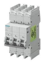
Miniature circuit breaker 240 V 10kA, 3-pole, D, 30 A, D=70 mm according to UL 489  $\,$
