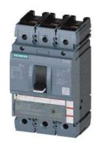
circuit breaker 3VA5 UL frame 250 breaking capacity class C 100kA @ 480 V 3-pole, line protection TM230, FTAM, In=100A overload protection Ir=100A fixed short-circuit protection Ii=5...10 x In nut keeper kit on both sides
