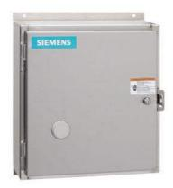
Non-reversing contactor, Size 2 1/2, Three phase full voltage, Contactor amp rating 60A, 3 wire (NO aux included), 110V 50Hz / 120V 60Hz coil, Non-combination type, Encl NEMA type 4X 304 S-Steel, Water/dust tight noncorrosive, Extra-wide enclosure
