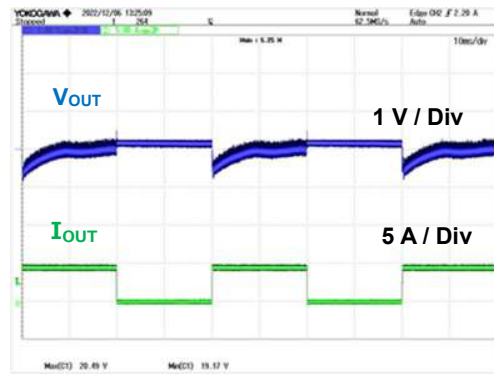
Figure 20. V_{IN} = 264 \text{ Vac} , I_{OUT} = \text{switch } 0 \text{ A} / 4.5 \text{ A}
