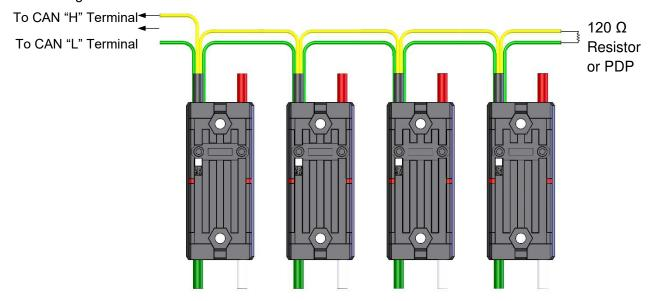
After all of the Talon SRXs have been wired, there will be 2 remaining signal wires – connect these two wires using a 120  $\Omega$  resistor or to the CAN interface on the Power Distribution Panel (PDP) to properly terminate the cable end.
