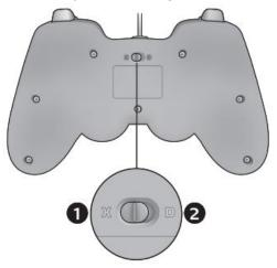
This is done because this allows the 'X' setting to serve as a reliable robot-disable or emergency-stop. In other words, selecting 'X' will be equivalent to unplugging the gamepad, which will zero all gamepad signals.
