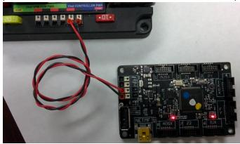
Alternatively the HERO can be powered using one of the PDP WAGO channels.
