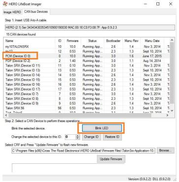
Then, in a moment, the device's status LED will rapidly blink. If the CAN device already has application firmware, it will rapidly blink **orange**. If the CAN device is in bootloader (perhaps the previous field-upgrade attempt was interrupted) then it will rapidly blink **green-orange**. Regardless of the state of the CAN device, it will respond in a unique fashion.
