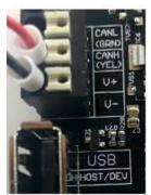
For robot applications that use 12V sources (such as lead-acid batteries or power supply) the Weidmuller press-insert connector can be used to connect  $V^+$  and  $V^-$ .
