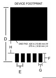
PINS ON .1 in CENTERS PROVIDE COMPATIBILITY WITH BREADBOARDS AND SOCKETS.
