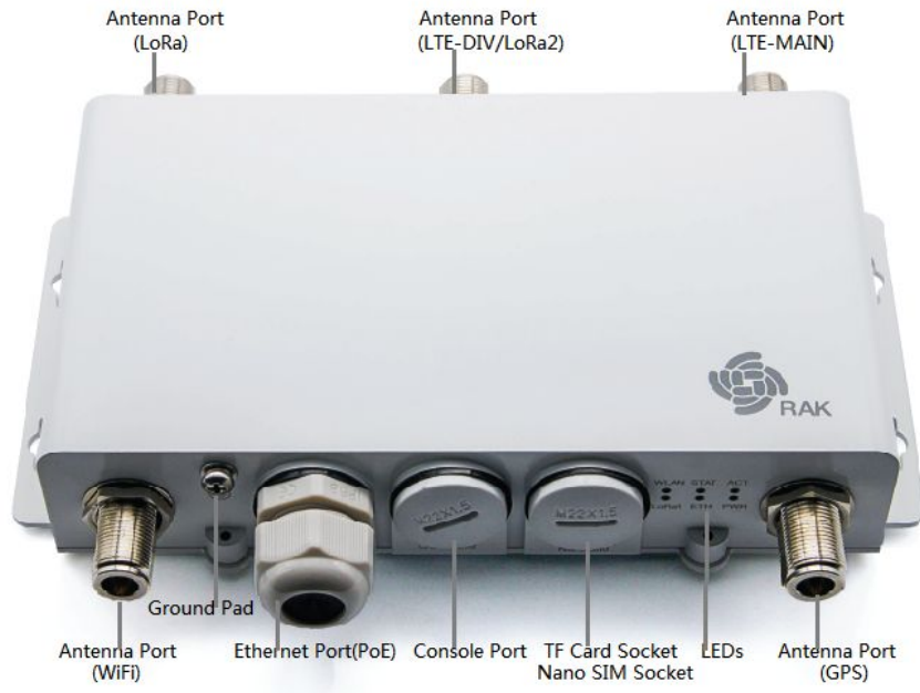
Figure 3: RAK7240 WisGate Edge Prime Hardware Interfaces
