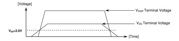
To prevent IC from malfunctioning,  $V_{\text{DISP}}$  should be applied after  $V_{\text{DD}}$  is applied. When turning off the power,  $V_{\text{DD}}$  should be applied after  $V_{\text{DISP}}$  is applied.
