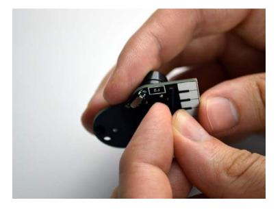
2. Place 3 nuts onto the 3 screws and tighten them down against the circuit board. These create the " piano legs".
