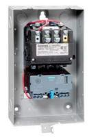
Non-reversing motor starter Size 1 Three phase full voltage Solid-state overload relay OLRelay amp range 0.25-1A 110VAC 50HZ / 120VAC 60HZ coil Combination type Indoor general purpose use
