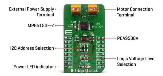
Its internal safety features include over-current protection, input over-voltage protection, undervoltage lockout (UVLO), and thermal shutdown. The MP6515GF-Z integrates four N-channel power MOSFETs with 2.8A peak current capability. It is designed to drive DC brush motors, solenoids, or other loads.
