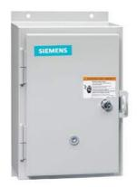
Non-reversing motor starter, Size 0, Three phase full voltage, Solid-state overload relay, OLRelay amp range 0.25-1a, 24VAC 50-60HZ coil, Non-combination type, Enclosure type 12, Dust/drip proof for indoors, Extra-wide enclosure
