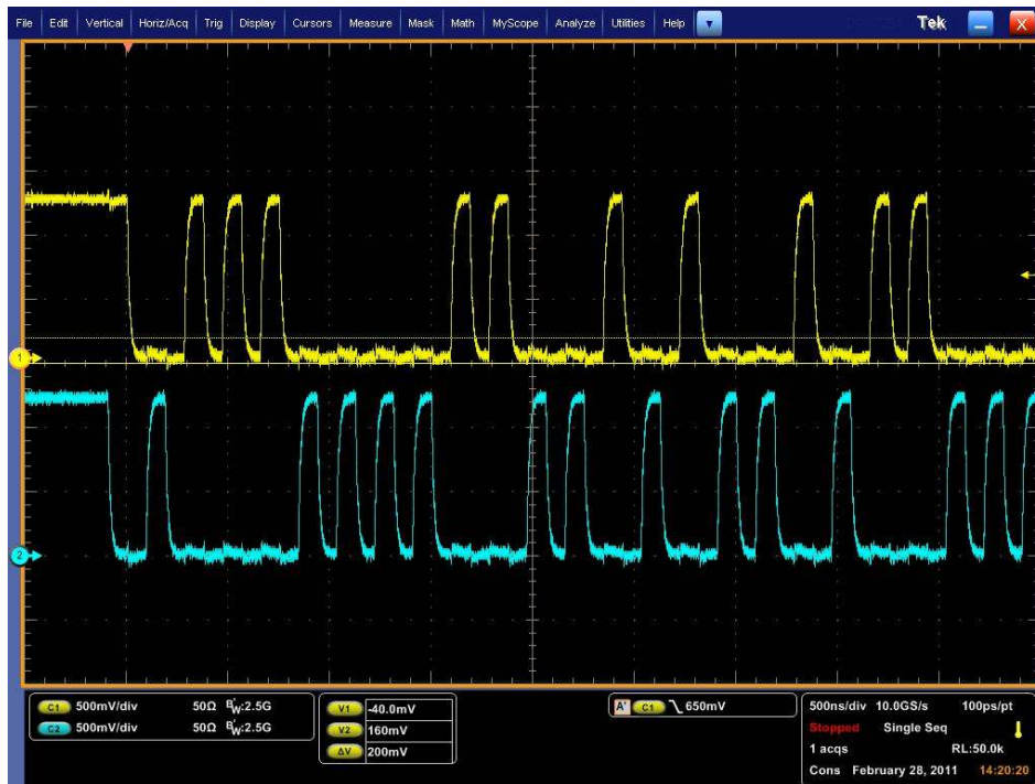
Figure 8. EMI4183MU MIPI D-PHY LP Mode Measured Results
