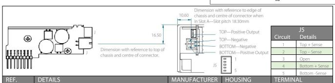
OUTPUT SIGNALS: 5 Pin, 1.25mm, with Friction lock, 28-32 AWG MOLEX 0510210500 0500588000
