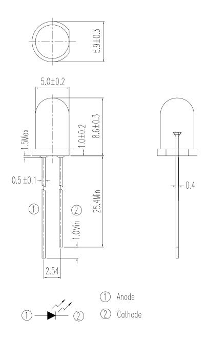
Note: Tolerances unless dimensions ±0.25mm
