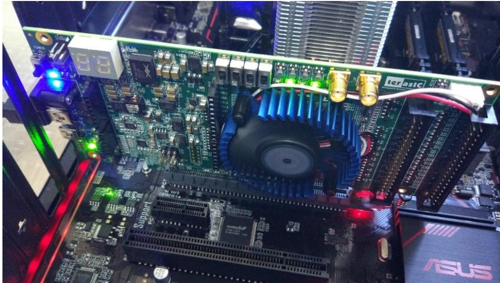
Figure 7-3 Install the FPGA board on the PC
