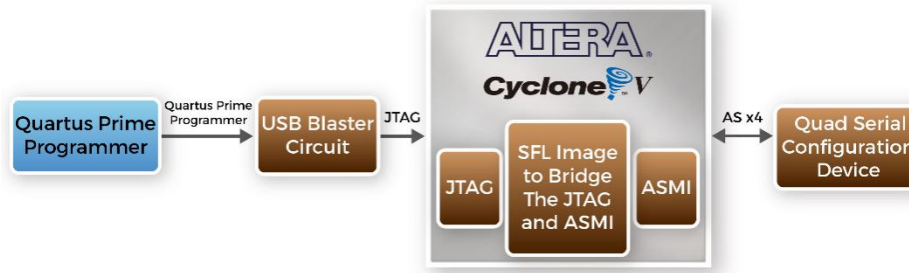
Figure 3-10 Programming a quad serial configuration device with SFL solution
