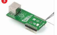
3. Plugging the board in Once you have soldered the headers board is ready to be placed into the de mikroBUS<sup>\*\*</sup> socket. Make sure to alig
