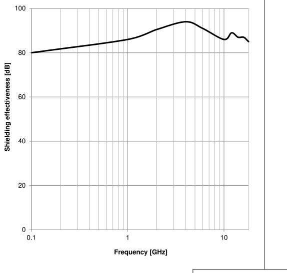
CHECKED REVISION DATE (YYYY-MM-DD) GENERAL TOLERANCE PROJECTION METHOD JoV 004.002 2019-01-01 DIN ISO 2768-1m DESCRIPTION **WE-LT Conductive Shielding** Würth Elektronik eiSos GmbH & Co. KG Gasket ORDER CODE EMC & Inductive Solutions Max-Eyth-Str. 1 30829048 74638 Waldenburg Germany SIZE/TYPE STATUS Tel. +49 (0) 79 42 945 - 0 www.we-online.com BUSINESS UNIT PAGE WÜRTH ELEKTRONIK 2/3 P-Profile eiSos Valid eiSos@we-online.com
