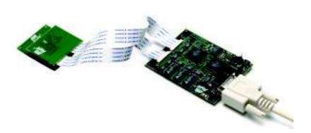
The AVR® ICE 200 In-Circuit Emulator is the perfect choice! A real-time In-Circuit Emulator based on a highly integrated AVR emulator chip.
