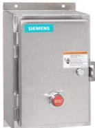
Non-reversing motor starter Size 0 Single phase full voltage Solid-state overload relay OLRelay amp range 3-12A 190-220/220-240V 50/60HZ coil Combination type Water/dust tight non-corrosive
