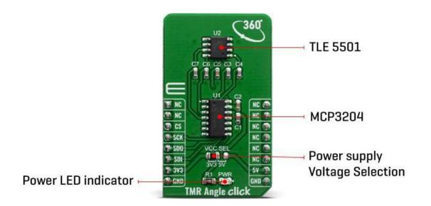
Some of its key features include large output signals of up to 0.37 V/V for easy analog value readout, discrete bridge with differential sine and cosine output, a very low supply current < 2.5 mA, a magnetic field range 20 mT to 100 mT and a Typ. angle error < 1.0° (over the whole temperature and lifetime profile). It has been primarily designed for safety.
