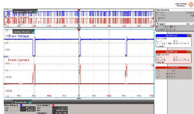
Figure 21 – Drain Voltage and Current Waveforms. 265 VAC, 800 mA Output. Drain Voltage: 150 V / div., 1 ms / div. Drain Current: 500 mA / div., 1 ms / div. Zoom = 10 \mu s / div. I_{DS(MAX)} = 1.66 A, V_{DS(MAX)} = 436.96 V.
