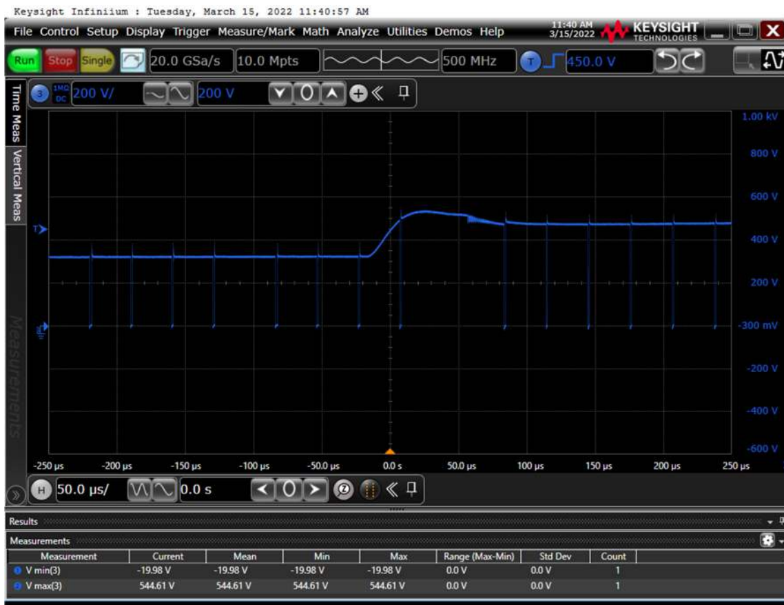
Figure 97 – Drain Voltage, 230 VAC, Full Load.
