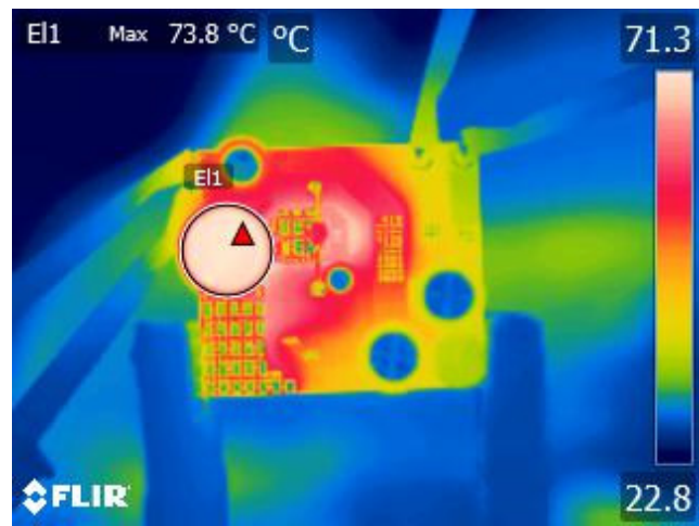
Figure 13 – Buck Choke (EI1), 73.8 °C. 265 VAC, 800 mA Output.
