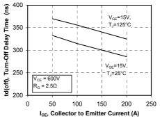
Turn-Off Delay Time vs Collector Current
