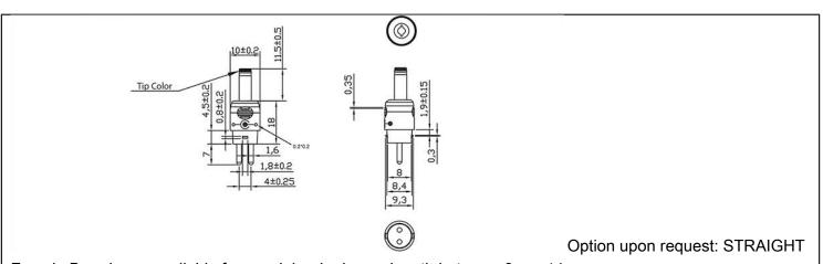
Female Barrels are available for special order in any length between 9mm-14mm This novel system allows for rapid shipment of prototype samples or small quantities of common output voltage and current which can fulfill the needs of most common barrel plug as well as male plug specs. The table explains the standard and non-standard options available as part of this system. This system also allows for both Center Positive and Center Negative polarity.
