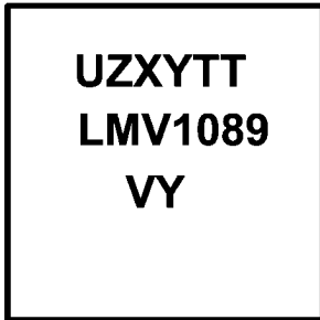
Top View U = Wafer Fab Code Z = Assembly Plant Code XY = 2 Digit Date Code TT = Die Traceability LMV1089 = LMV1089VY
