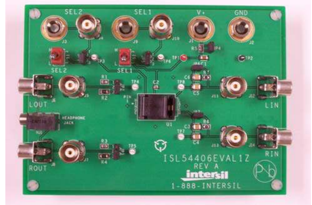
FIGURE 1. ISL54406EVAL1Z EVALUATION BOARD
