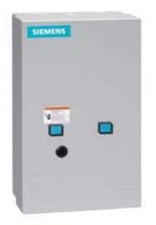
2-speed 3-phase motor starter, Size 0, Two separate windings, Constant horsepower, Solid-state overload relays, Low Spd OLR range 0.75-3.4A, High Spd OLR range 3-12A, 24VAC 50-60Hz coil, Enclosure NEMA type 1, Indoor general purpose use
